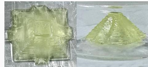
Figure 1: 3D PEG hydrogel printed from precursor solution of JenKem® 8ARM(TP)-ACLT-10K, and M-QTX.
